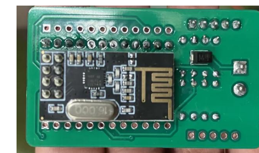
Figure 3a: nRF24L01 PCB in Battery Chamber
