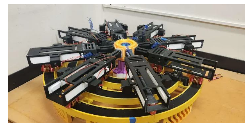
Figure 1c: Battery Vending Machine Prototype
