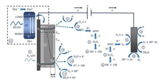
Here, the hydroxyl radicals (OH•) are generated at the surface of the photoelectrode and can subsequently participate in various chemical reactions, including the oxidation of pollutants and greenhouse gases, thereby contributing to the cleansing of the atmosphere.
