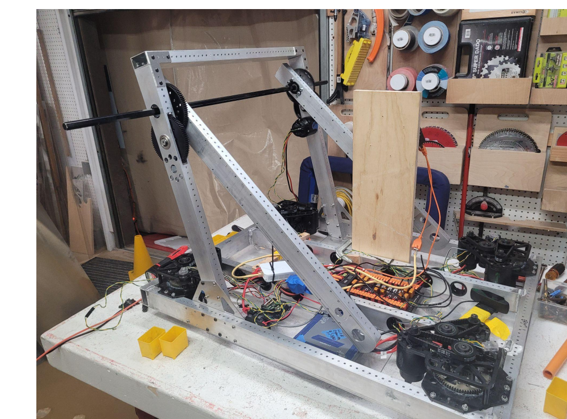
Step 4: Create the basic framework of the robot. The wooden board in the picture is to test the range of the robot's camera. The wooden board is used because the height and angle of the camera can be better adjusted.
