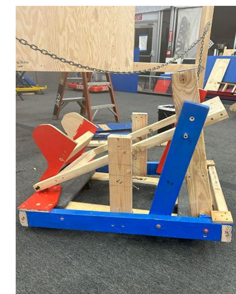
Step 2: Make the rough outline and parts of the robot out of wood. The advantage is that it can improve fault tolerance and reduce costs.
